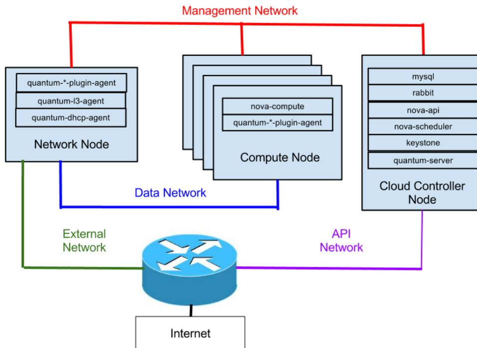
A standard Quantum setup has up to four distinct physical data center networks:
